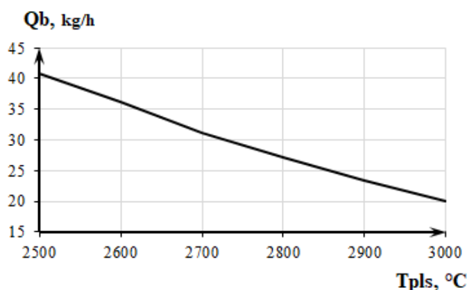
Fig. 8. Calculated dependence of water consumption on the average mass temperature of the plasma jet
